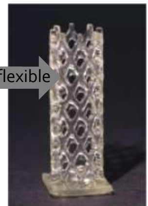
Figure 2: Stent-like structures with memory effect
