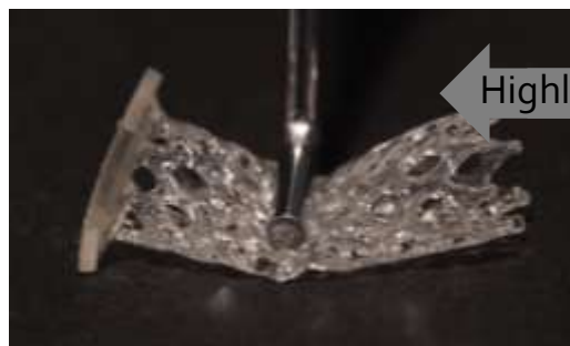
Figure 2: Stent-like structures with memory effect
