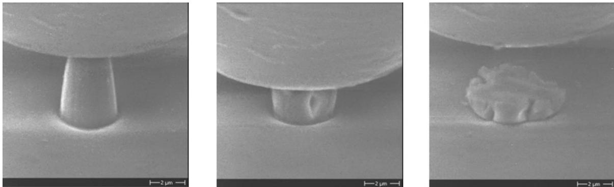
Figure 1 : In Situ SEM compression of a fused silica micropillar
