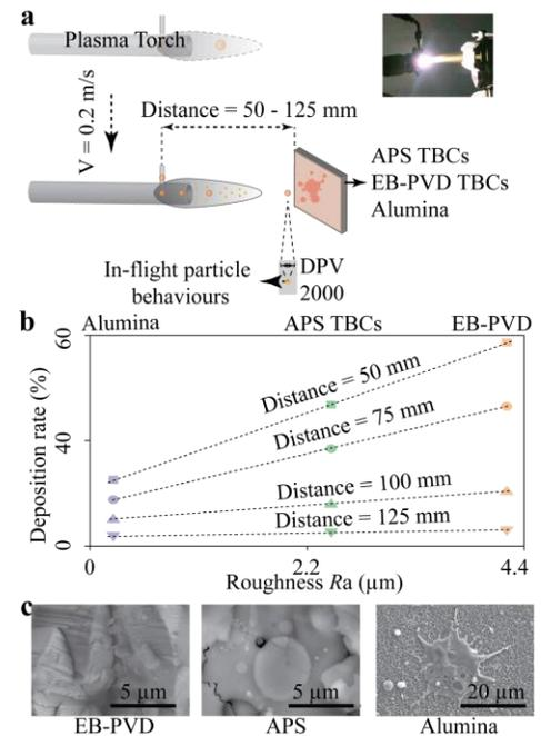
Figure 1. (a) A schematic of the experimental setup for capturing initial formation of molten volcanic ash layer under plasma spray conditions. (b) Roughness-deposition rate relationship for EB-PVD TBCs, APS TBCs and alumina substrate under different distance to nozzle, (c) The morphology of splats onto various substrates.
