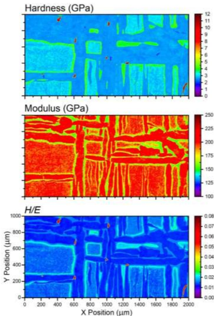
Figure 1 – Nanoindentation maps of the Hardness, Modulus and H/E ratio of a region of the Taza meteorite showing Kamacite bands in a Plessite matrix.
