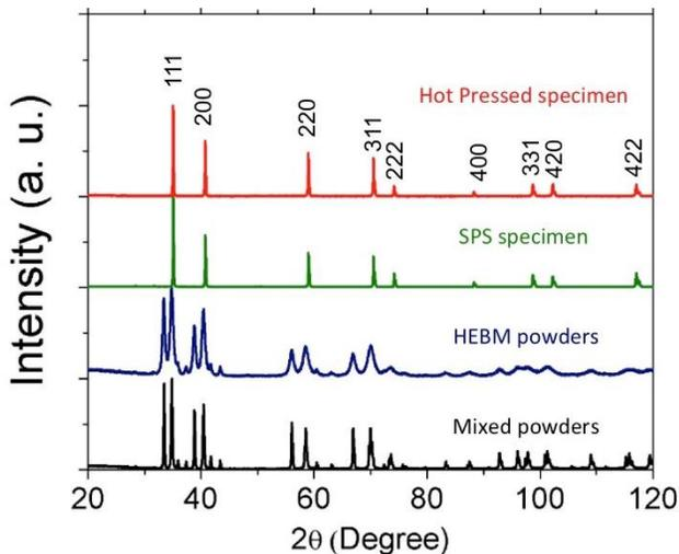
Figure 1 – Experimental X-ray diffraction patterns of a  $(\text{Hf}_{0.2}\text{Nb}_{0.2}\text{Ta}_{0.2}\text{Ti}_{0.2}\text{V}_{0.2})\text{C}$  following each processing step, starting with hand mixed powder, to high-energy ball milled powder, to sintered specimen, and finally hot press annealed specimen, demonstrating the progression into a single phase.
