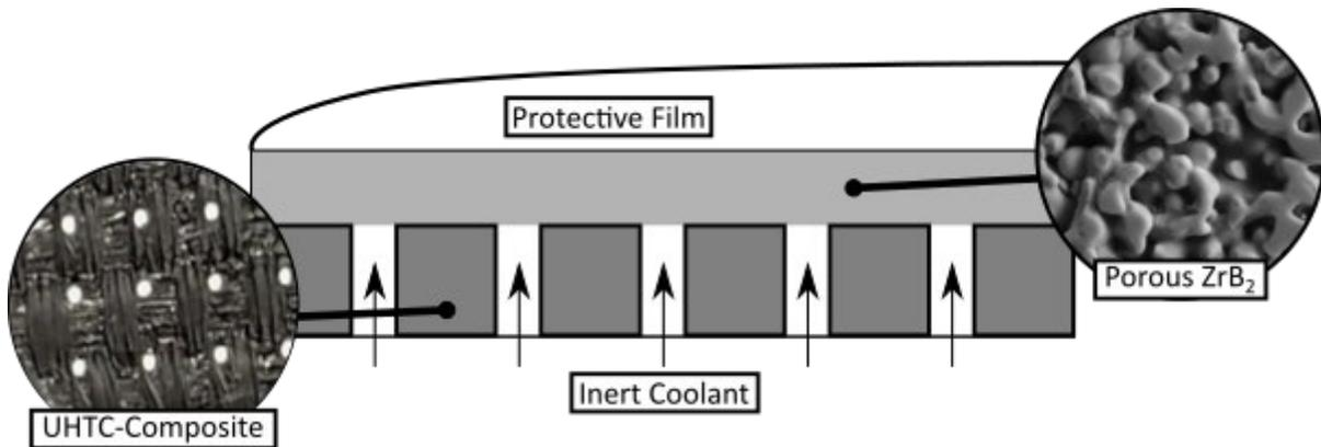
Schematic of a transpiration cooled UHTC system. Porous partially sintered  $ZrB_2$  sits above a channeled substructure of ceramic matrix UHTC composite. Coolant gas flows through the system, creating a boundary layer that protects from oxidation.
