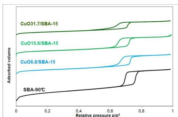
Figure 1: N<sub>2</sub> physisorption isotherms of the parent support and of the adsorbents. For a better visibility the isotherms are shifted along the Y axis.
