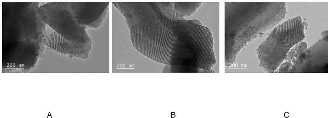
Figure 2: TEM micrographs (A, B and C) of the fresh adsorbents CuO8.8/SBA-15, CuO15.6/SBA-15 and CuO31.7/SBA-15 respectively.
