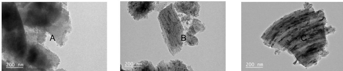
Figure 4: TEM micrographs (A, B and C) of the aged adsorbents (after SO<sub>2</sub> adsorption tests) CuO8.8/SBA-15, CuO15.6/SBA-15 and CuO31.7/SBA-15 respectively.
