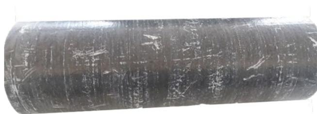
Figure 2 : Proof of concept in PyroKarb made by filament winding
