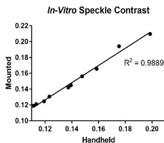
Figure 2 - Speckle Contrast Values within Flow Region Using Mounted and Handheld Setup. Flow speeds between 0-5 mm/s.
