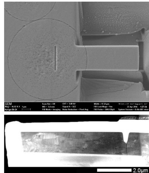
Figure 1 – Examples of pre- and post-testing microcantilevers.
