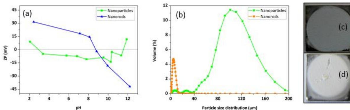
Figure 1: Zeta potential (a) particle size distribution (b) for suspensions of nanoparticles and nanorods; surface morphology of SnO<sub>2</sub> films deposited with nanorods (c) and nanoparticles (d) and sintered at 500 °C for 2 h.
