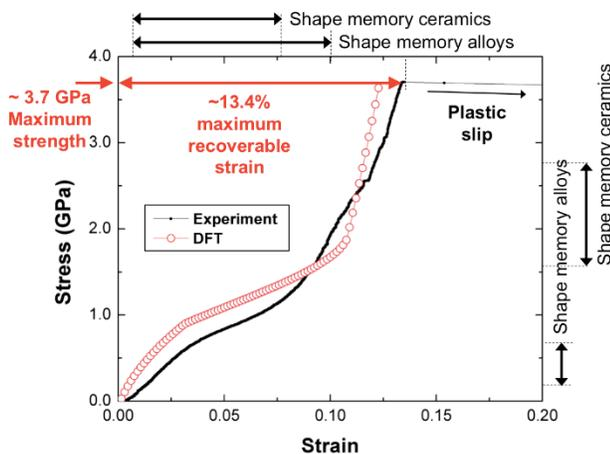
Figure 1 – Stress-strain curve of  $[0\ 0\ 1]$   $\text{CaFe}_2\text{As}_2$  single crystal
