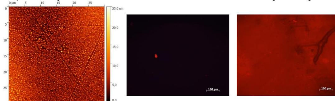
Figure 1 - AFM image of a PVCL/MEA 20 microgel film (left), fluorescence microscopy image of a PVCL/MEA 20 microgel film after incubation with tetramethylrhodamine-BSA (middle) and pure glass after incubation with tetramethylrhodamine-BSA as reference (right).
