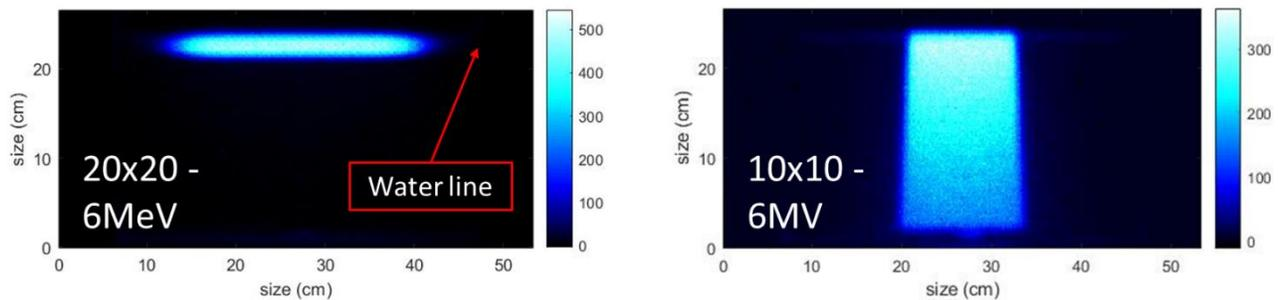
Figure 1: Water tank phantom images with different beam parameters. Left: 20x20cm electron beam, Right: 10x10cm X-ray beam.
