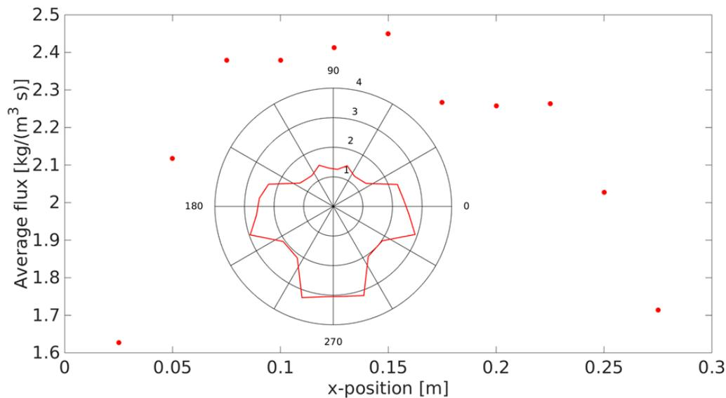
Figure 2: Volumetric hydrogen fluxes in  $\text{kg}/(\text{m}^3 \cdot \text{s})$  at various  $x$ -positions and angles in a fluidized bed with a horizontal staggered membrane set-up.
