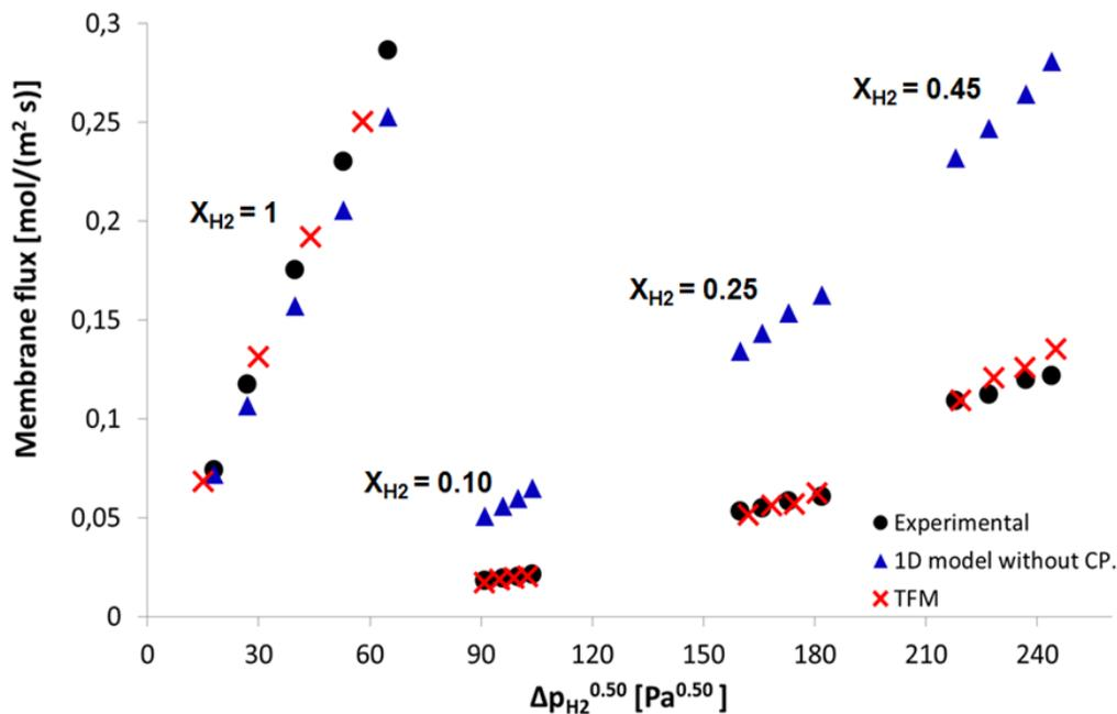
Figure 1: Hydrogen membrane fluxes at various hydrogen inlet fractions for the vertical membrane set-up.
