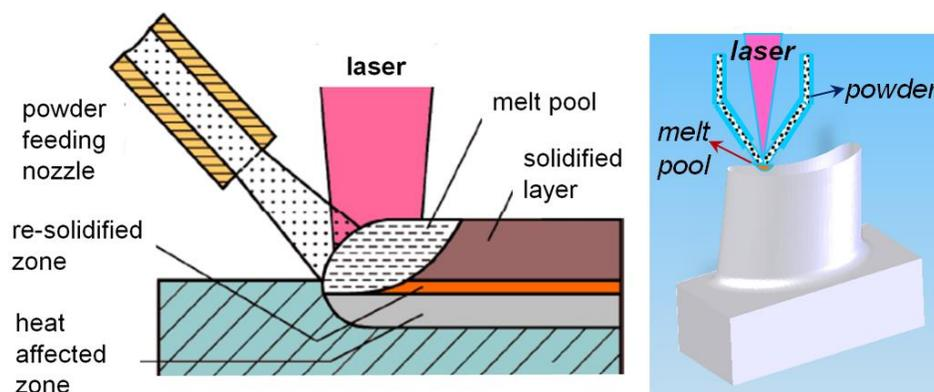
Figure 1 – Schematic diagram of power feeding laser additive manufacturing process
