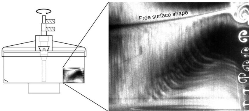
Figure 1 - An example of Taylor-Görtler vortices formed at the wall of a mimic of the CentriCult™ unit during spin-down to rest, visualised with fluorescent rhodamine dye
