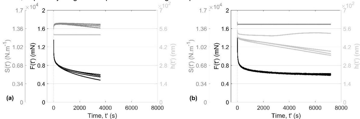
Figure 1 – Two sets of four relaxation tests performed on PMMA.  $t'$  is considered as the time from the beginning of the hold segment. (a) Displacement is maintained constant during one hour and significant discrepancies appear in load and contact stiffness measurements. (b) Contact stiffness is maintained constant during two hours. Drift can be directly estimated through displacement measurements and no discrepancies can be seen on load signal.
