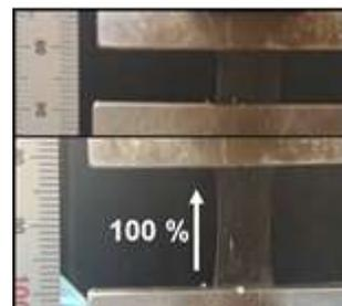
Figure 1 Photo of tensile test of TFA/Ag nanowire composite
