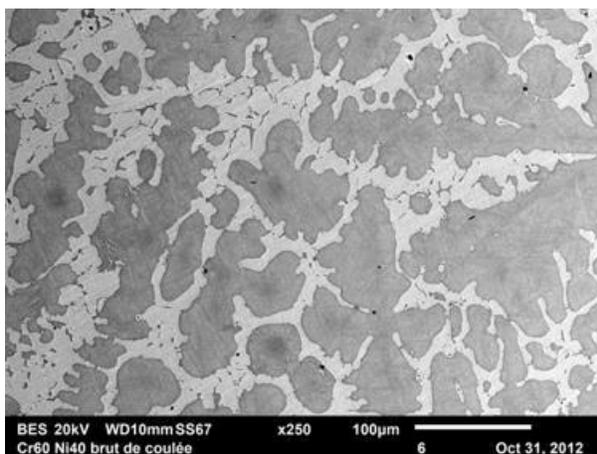
*Figure 1– As-cast microstructures of one of the cast Cr-Ni alloys (SEM/BSE)*
