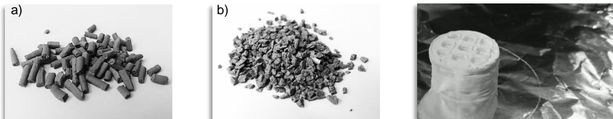
Figure 1 - Formulations of: a) binder-containing extruded pellets, b) binderless compressed granules and c) 3D-printed structures
