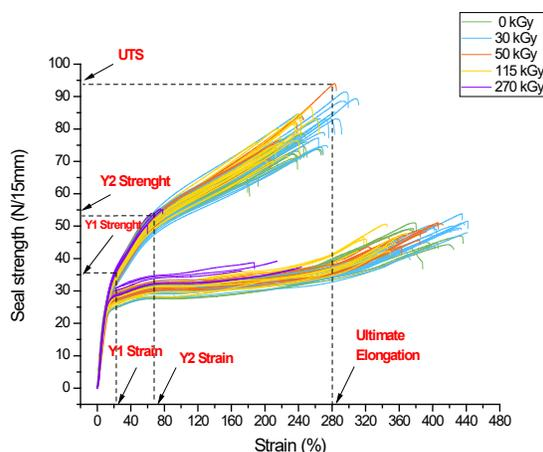
Figure 2: Strength-strain curves for each welding location (1-5) and each gamma doses (0-270 kGy) of EVA bag. Colors according to gamma doses.
