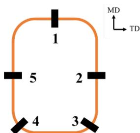
Figure 1: Five welding locations. Black lines correspond to welding samples (1-5). Orange lines correspond to welding.
