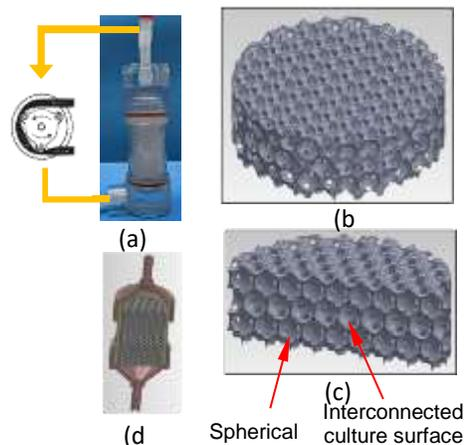
Figure 1 - (a) Pump driven continuous perfusion 3D bioreactor. (b) The 3D bioreactor matrix. (c) Matrix cross-section (d) Assembled bioreactor.
