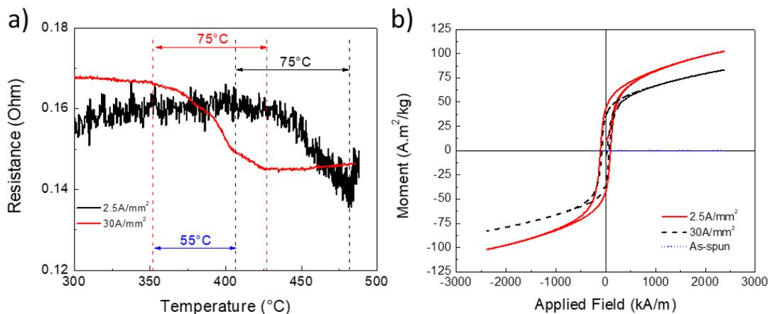
Figure 1 – Resistance change vs. temperature (a) and magnetic properties of the electrically annealed samples (b), as a comparison, the initial state (as-spun) is also shown.
