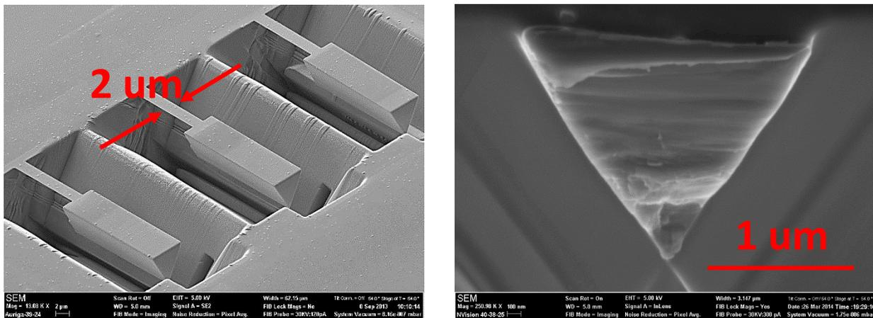
Figure 1 (a) Three micro-fatigue testing specimens prepared by focused ion beam; (b) fraction surface of one micro-fatigue cantilever after  $10^6$  cycles
