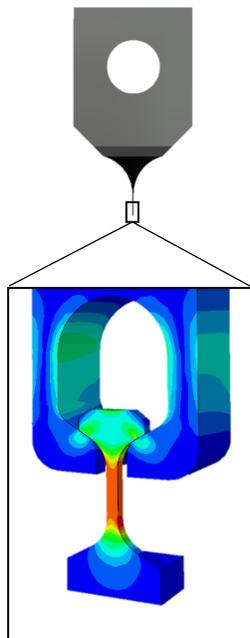
Figure 1 – Silicon gripper (top) and dumbbell bone sample (bottom)
