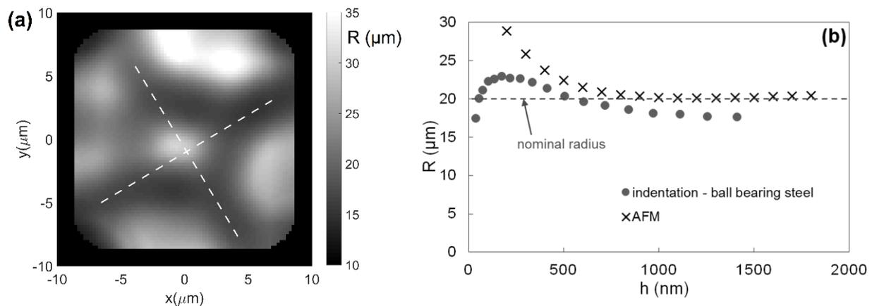
Figure 1 – (a) Local radius of spherical indenter with nominal radius 20  $\mu\text{m}$  (dashed lines show the four-fold symmetry of used diamond crystal) and (b) change of the radius with the distance from the apex obtained by AFM and by indentation on reference materials.
