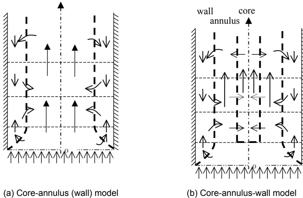
Figure 2 Heterogeneous flow structures in CFB.
