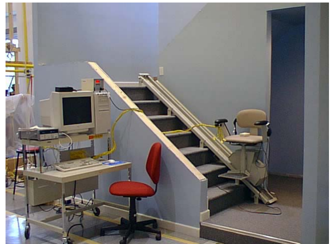
Figure 5. a) Competitive Assessment test station and b) electric stairlift undergoing competitive assessment testing.
