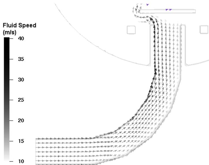
Figure 3: Vectors of gas velocity in the feed pipe
