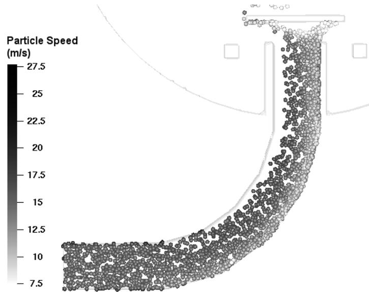
Figure 2: Particles colored by speed in the feed pipe
