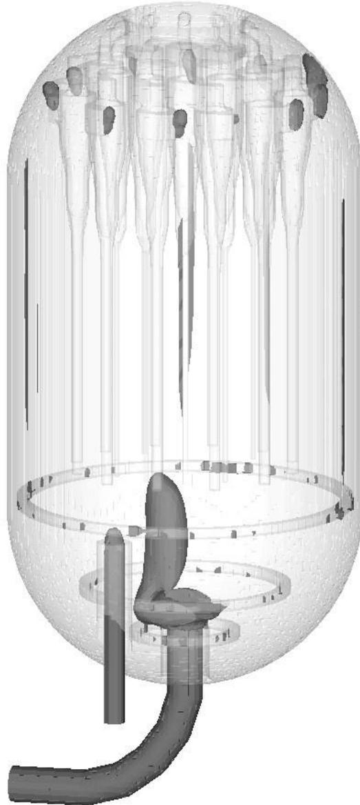
*Figure 4: Isovolumes of regions with gas velocity higher than 5 m/s*
