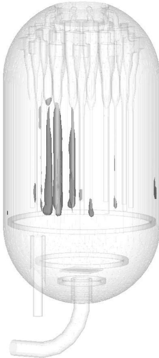
*Figure 5: Isovolumes of regions with high predicted wear due to particle impact*
