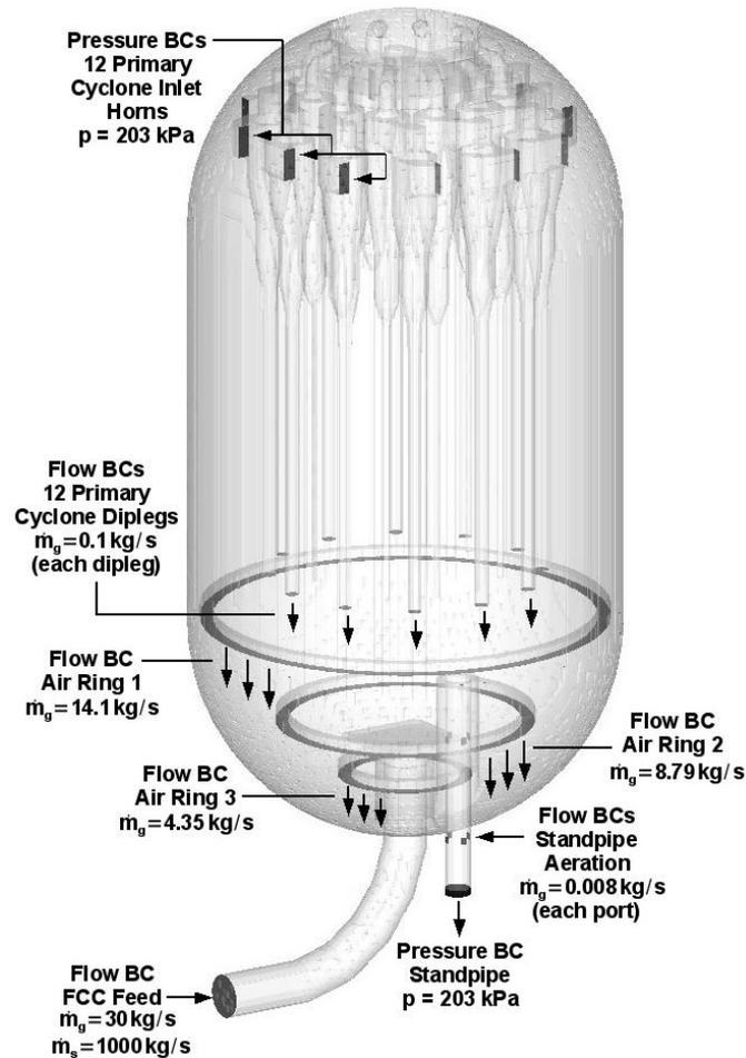
Figure 1: Geometry and boundary conditions for the FCC regenerator
