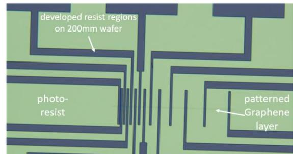
Figure 2: Patterned graphene test structure on 200mm wafer.
