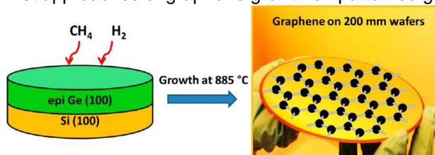
Figure 1: Germanium substrate realization and graphene synthesis on 200mm wafer (2).
